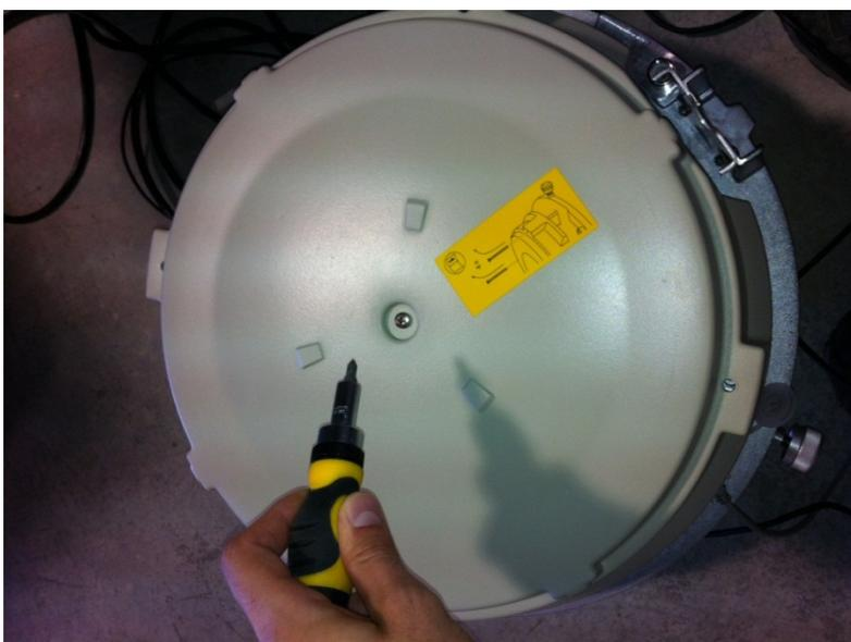
OTT Pluvio 2 Base with load cell plastic cover about to be removed
