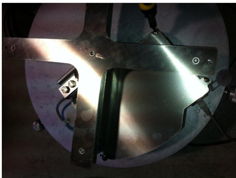
OTT Pluvio 2 terminal cover being removed
